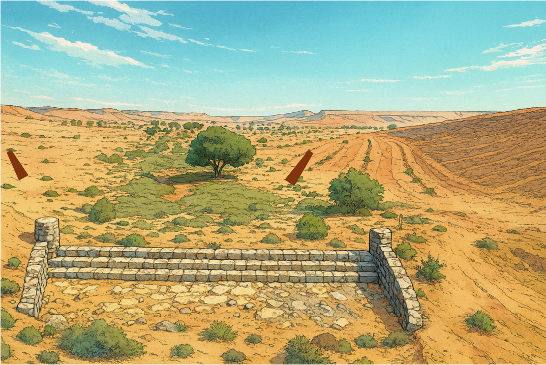
Figure 7. Design of a cross-wadi wall: after, you add the two wing-walls (brown) (© FAO/Éric Lacroix).
